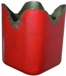
Square Deep Drawing Cup Test
