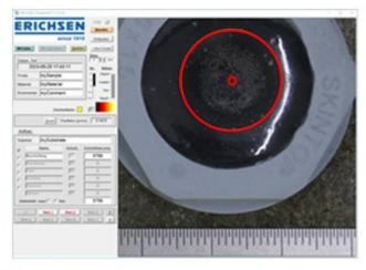
Several (up to 6) layers can also be marked and measured simultaneously.
