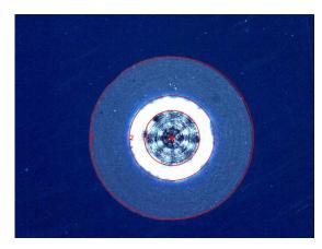
Depending on the drilling angle, by a tangential function the selected intervals can now be assigned due to the respective layer thickness of the obliquely vertically cut areas.
