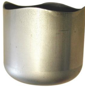
Deep Drawing Cup Test
